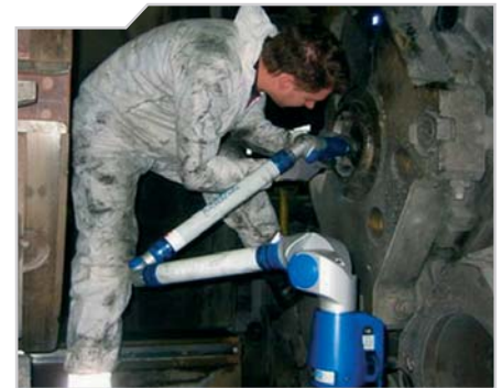
In-situ measurements with the measuring arm
