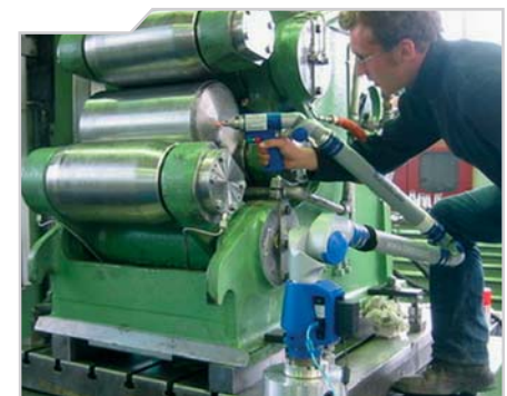
Checking the rolls of a roller mill with the measuring arm
