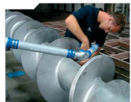
Control of a screw-conveyor
