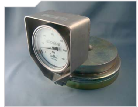
Type LPM between abutment and distribution plate
