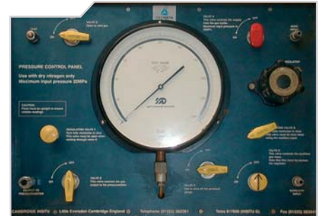
Control unit for gas-operation
