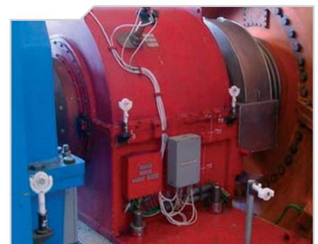
Prisms for monitoring a power-generating machine
