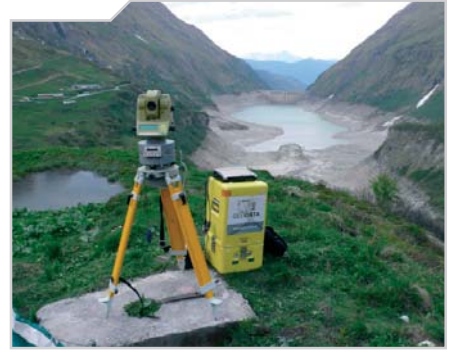
Calibration measurement for a hydro-power project
