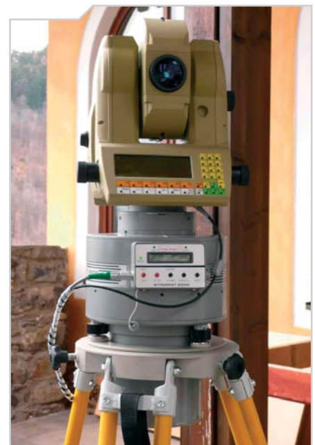
Gyromat 2000 with fix assembled Total-station
