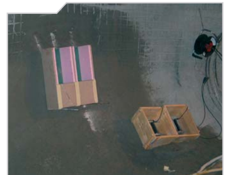
Formwork for making the specimen (left) and for the shrinkage test (right)
