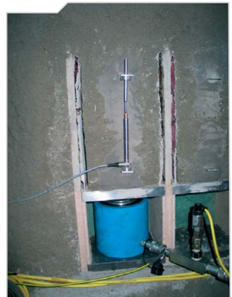
Test set-up with hydraulic cylinder and displacement transducer on specimen
