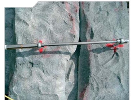
Joint meter with electric displacement transducer
