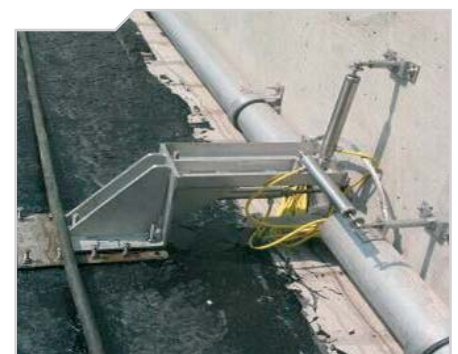
3D-joint meter in special design and for automatic data acquisition
