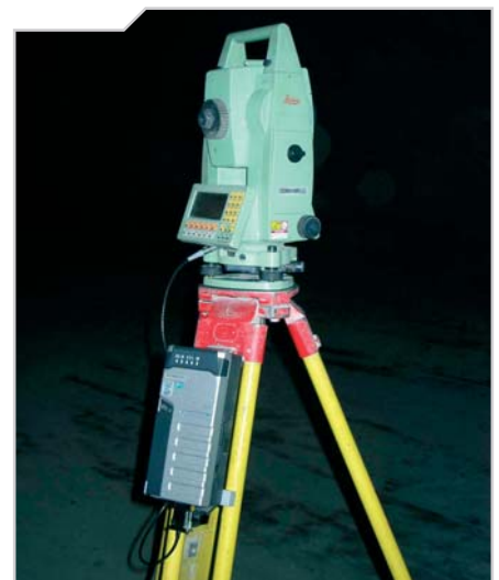
Totalstation with PC on tripod
