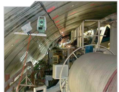
Motorised totalstation on console
