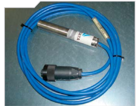
Pt 100 sensor with cable
