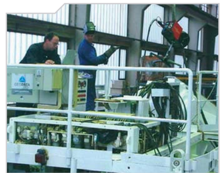
Installation of the guidance system for a road header in the manufacturing plant
